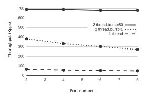
Figure 2: Forwarding performance of the optimized Open vSwitch code depending on the number of ports attached to the switch.
