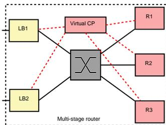
Fig. 1. Example of the multi-stage router composed by two load balancers and three back-end routers: all internal elements run on a different PC to improve performance and reliability.
