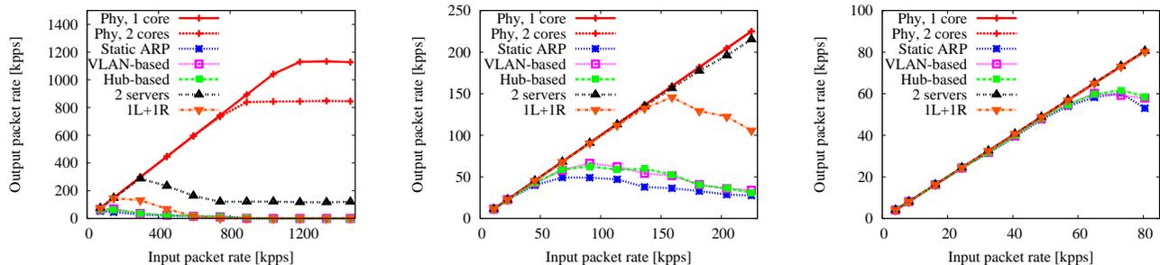
Fig. 3. Performance evaluation of multistage router (2 LB + 2 OSR) into VMware ESXi 4.0 environment with different internal configurations: from left to right, 64, 512 and 1500 bytes packets.
