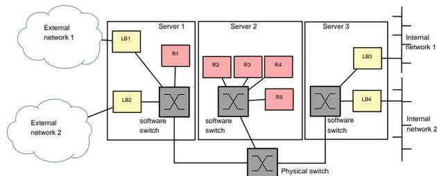
Fig. 2. Use case for introduction of virtualization in multistage router architecture: three physical servers hosts different virtual machines which are used to build up one or more virtualized multistage routers.
