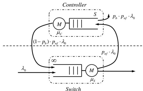
Fig. 1. A simple model of an OpenFlow switch.
