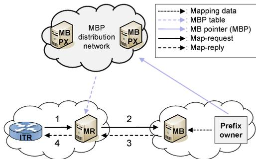
Figure 2: Basic structure and operation of FIRMS.
