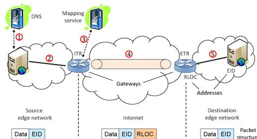
Figure 1: Locator/Identifier Separation Protocol.
