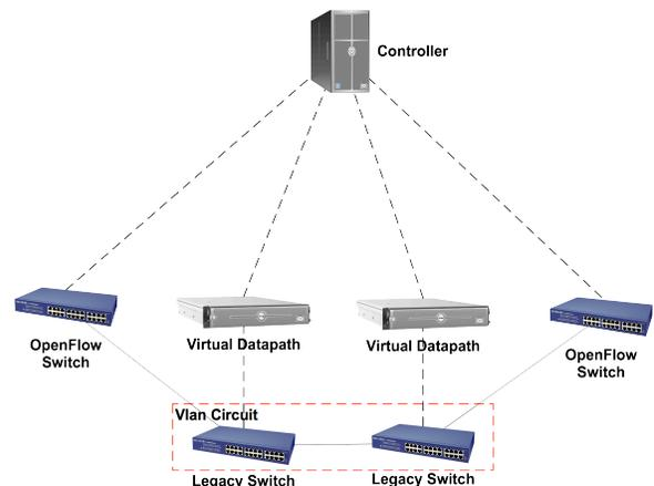
Figure 1. Openflow network is using the LegacyFlow solution.
