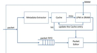
Fig. 1. Core module of the Smart Switch.
